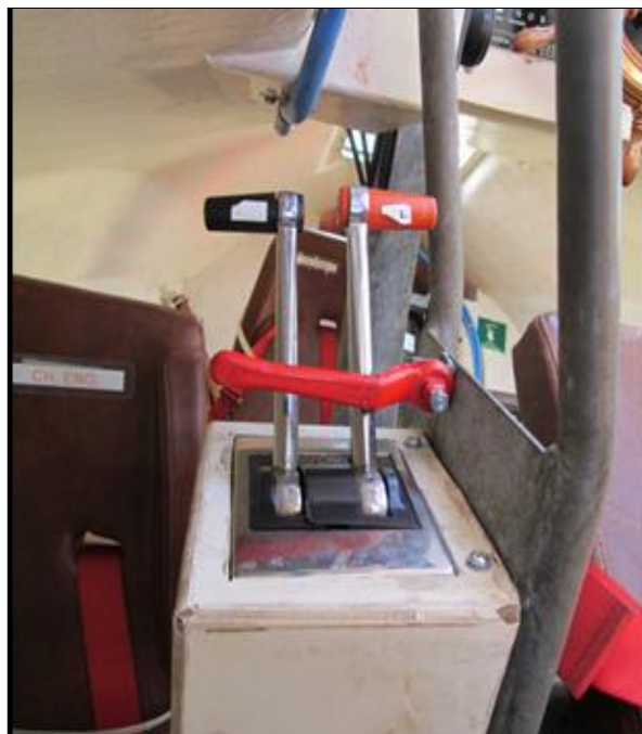
Figure 9. Safety device on NORDIC NORA
