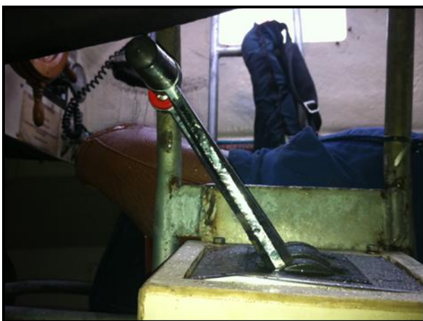
Figure 7 showing the security and release handles in the released position.
