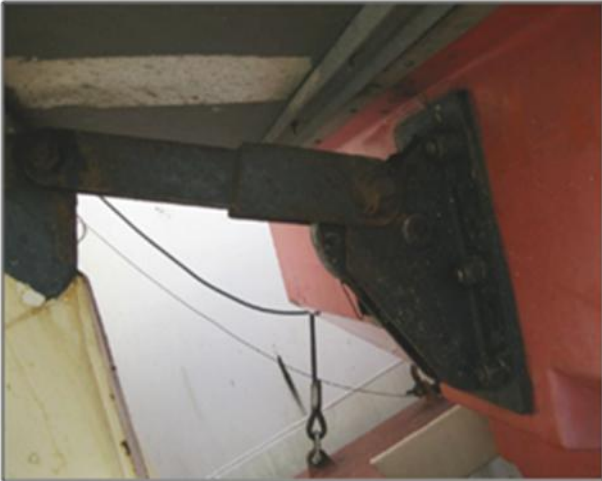
Figure 4 Boat mooring with release hook
