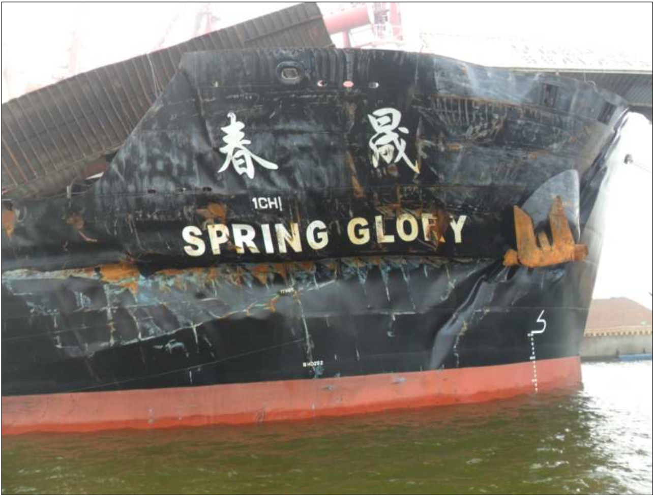
Figure 10: Damage to SPRING GLORY Source: Jiangsu Huaxi Ship Management Co., Ltd.
