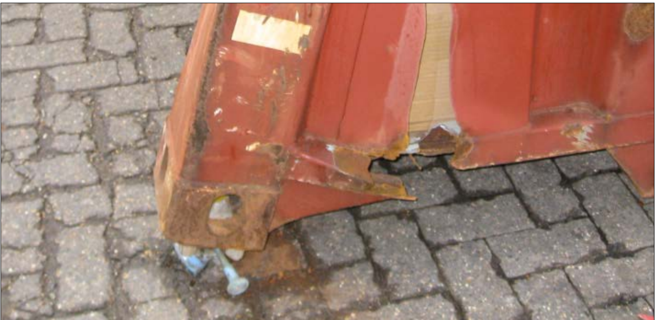
Figure 7: Damaged container Source: Maersk Line A/S
