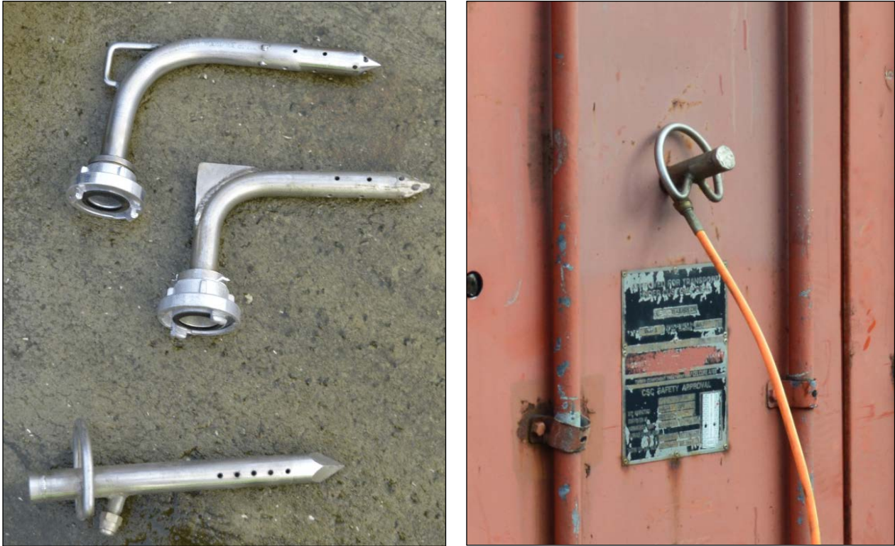
Figure 10: Firefighting spear nozzles – Left: Two water spears, one CO 2 spear. Right: CO 2 spear mounted in container. Source: DMAIB
