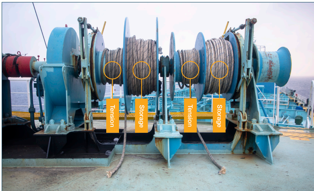
Figure 6: Combined windlass and double split drum mooring winch.
